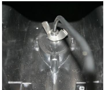
12. When the Signal Booster is fitted the plug for the sonar should be facing forward.
