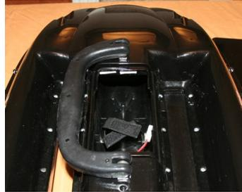
2. Remove the screws from the wireless sonar cover underneath.
