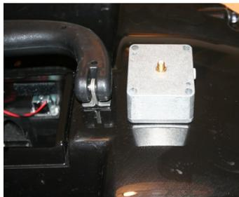
13. Using masking tape mark up where the hole will be drilled for the aerial. This should be 100mm in front of the handle.
