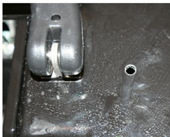
17. Run a small bead of silicone in a circle around the aerial fitting on the booster box.
