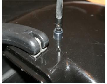
21. Leave the boat for 24 hours in a horizontal position to allow the silicone to fully dry/cure.
