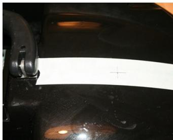
14. You will need to remove the cable tie for the LED wiring before drilling the hole. The box should be mounted this far forward to reduce electrical interference from the boats components.
