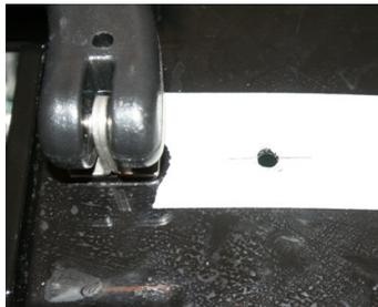
16. Remove the masking tape and clean any burrs from the hole both inside and out.
